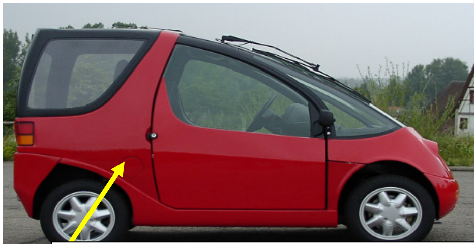
Lid for charging: battery charger for Solar & 220 Volt-net in it
